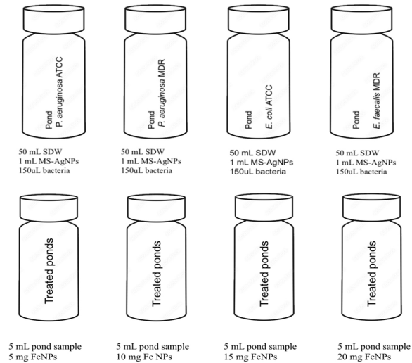
Figure 2. Water treatment setup using MOS-Fe 3 O 4 NPs for the removal of residual Ag NPs and microbial debris. Treated samples were incubated with varying FeNP concentrations, vortexed, and analyzed for turbidity and removal efficiency.
