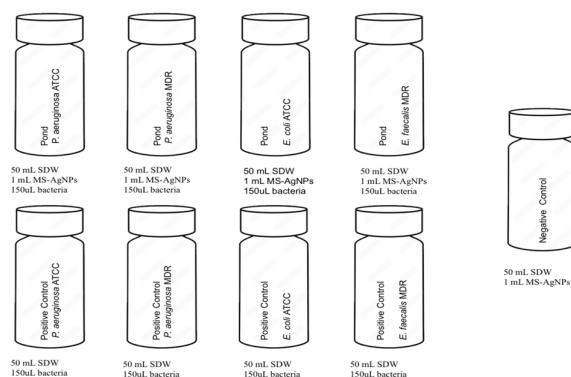
Figure 1. Experimental setup for antibacterial testing of MOS-Ag NPs. Each synthetic water sample, standardized bacterial inoculum, and MOS-AgNP suspension. Positive and negative controls were included.
